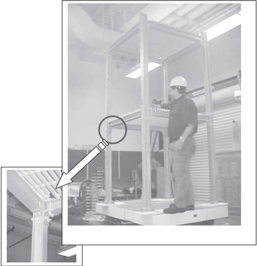
Figure 7-76. Seismic evaluation of 3-D FRP frame structure with FRP gratings. Source: Mosallam (2000).
