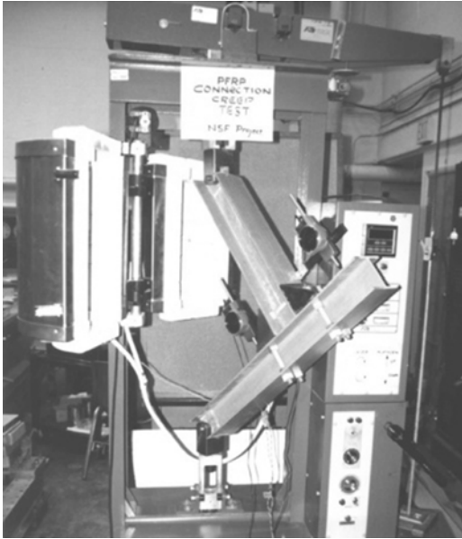
Figure 7-49. PFRP connection creep test setup.
